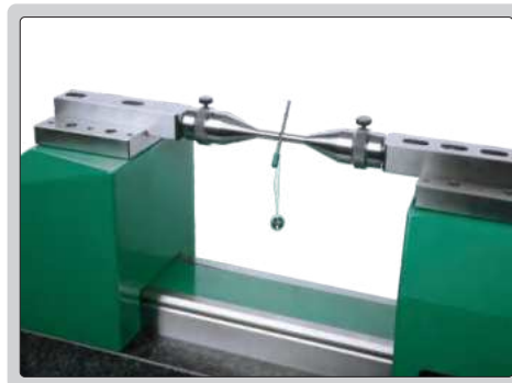
pin gauge measurement
