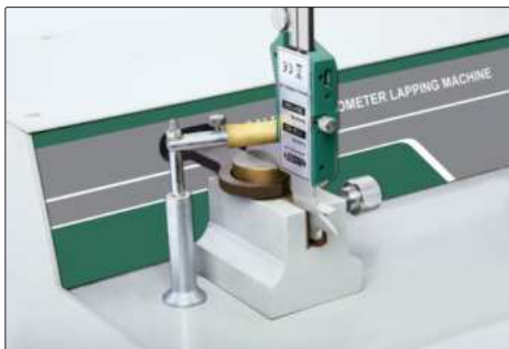
lapping measuring surfaces of caliper lower jaws
