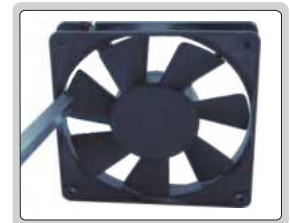
measuring blade to sidewall gap
