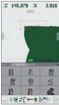
fast measurement, automatic recognition of cutting edge shapes
