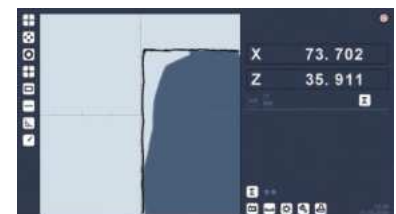
scanning the maximum profile of cutting tools
