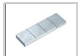
stainless steel plate test block (included)
