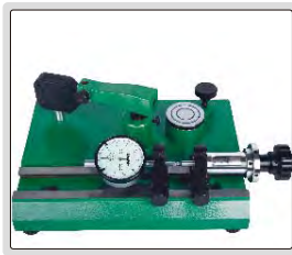
inspect accuracy of dial indicators (range 0-25mm)
