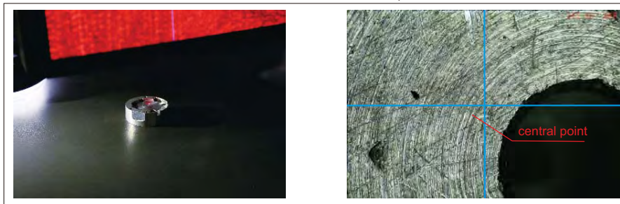
laser indicator locates the central point
