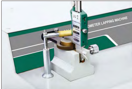
lapping measuring surfaces of caliper lower jaws
